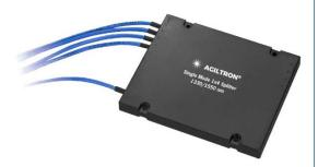
This FC Series fiber optic coupler provides monolithically integrated 1x4 function in a compact format. It features good uniformity, low excess loss and very low polarization sensitivity. The device is ideal for splitting or combining light with exceptional performance over a wide wavelength range.
